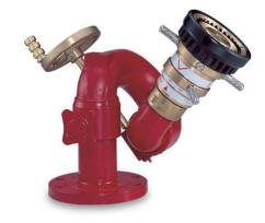
Siv is a 3" monitor for fixed installations made of corrosion resistant bronze, with an unobstructed 3" waterway for low friction loss and high flow. It is suitable for water and foam applications both onshore and offshore. It has been approved by Lloyds register for marine use.
